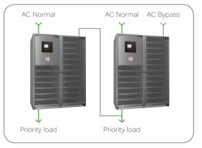
Parallel connection for increased power with a centralized bypass unit and up to 8 UPS units
