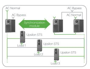
Distribution redundancy with the Static Transfer Switch (Upsilon STS)
